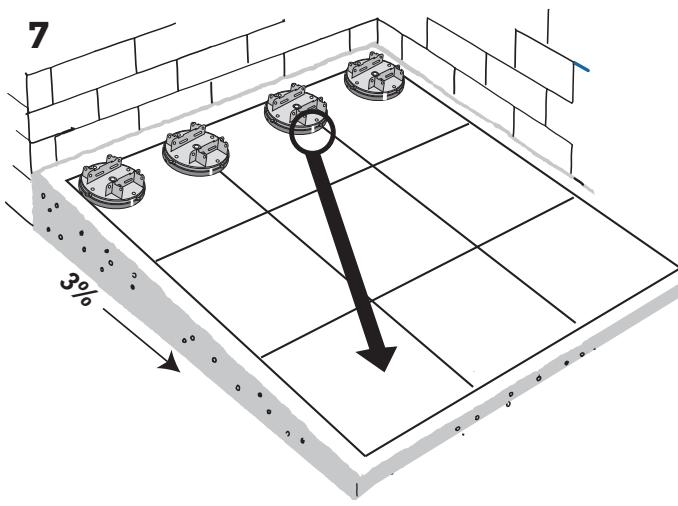
Use the DPH-F17 and DPH-F28 pedestal on the first line because they are not adjustable in height for the following lines
